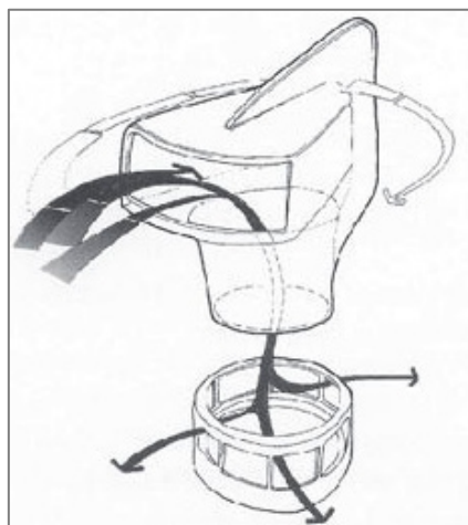
Figure 17 Schematic drawing of a supply air windscoop. 13
