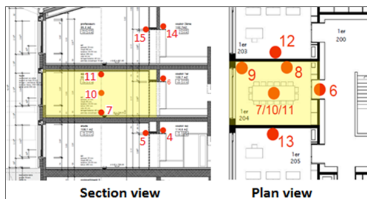
Figure 56 Overview of temperature sensor locations in and around the monitored room.
