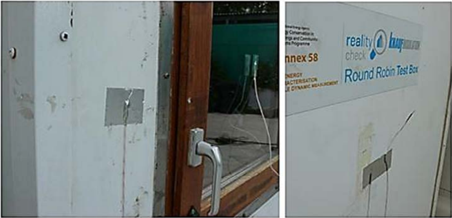
Figure 60: Assembly of the instrumentation in the exterior of the test box
