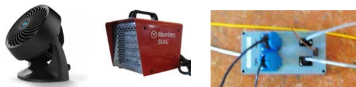
Figure 88: Advantech ADAM4011 module with electric fan and heater
