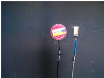
Figure 40: Installation of internal heat flux density and surface temperature sensors. First glued to the internal surfaces and then covered with a tape of same colour of the internal surface.
