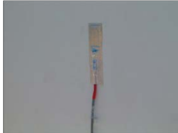
Figure 41: Installation of external surface temperature. First glued to the external surfaces and then covered with a tape of same colour of the external surface.
