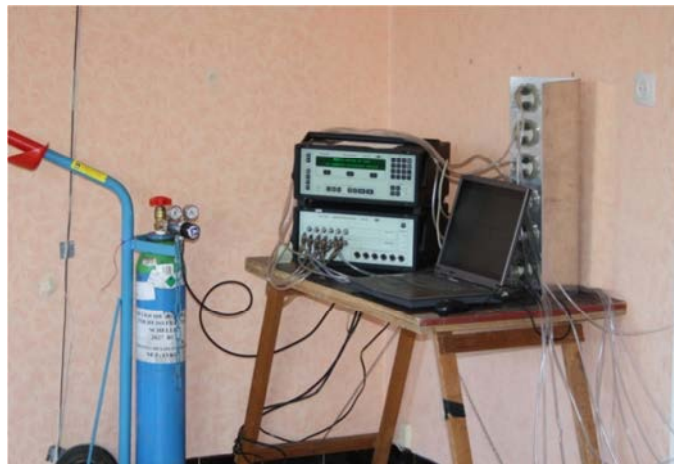
Figure 91: Tracer gas test equipment (here mounted in another investigated building)
