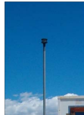
Figure 42: Meteorological sensors near the test box: Outdoors air temperature, global vertical solar radiation, wind speed and direction.
