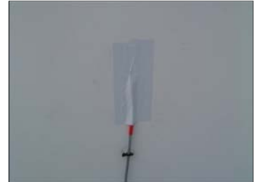
Figure 41: Installation of external surface temperature. First glued to the external surfaces and then covered with a tape of same colour of the external surface.
