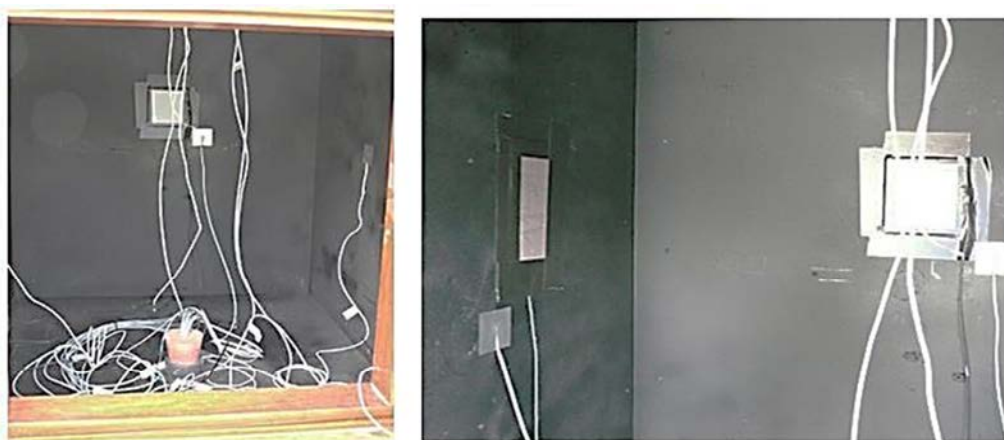
Figure 59: Assembly of the instrumentation in the interior of the test box
