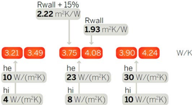
Figure 20: Effect on the calculated overall heat loss coefficient of the round robin box of both uncertainty on the fabric resistance as well as on the surface heat transfer coefficient.
