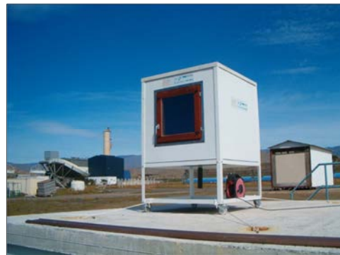
Figure 37: Placement. Facing south in an open area.
