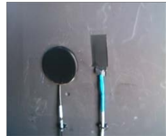
Figure 40: Installation of internal heat flux density and surface temperature sensors. First glued to the internal surfaces and then covered with a tape of same colour of the internal surface.
