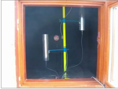
Figure 39: Indoors air temperature and shielding devices
