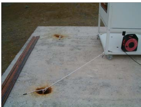
Figure 38: Anchoring additional to the brakes, to prevent damage due to strong winds which are very frequent in the test site
