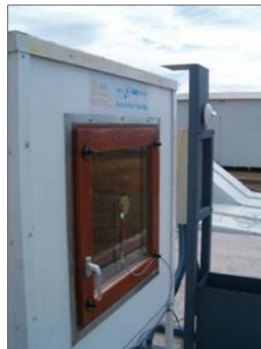
Figure 42: Meteorological sensors near the test box: Outdoors air temperature, global vertical solar radiation, wind speed and direction.
