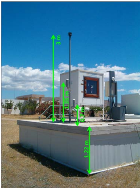
Figure 43: The test box and meteorological devices near to it (left), meteorological devices at meteo 1 (right)
