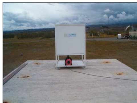
Figure 38: Anchoring additional to the brakes, to prevent damage due to strong winds which are very frequent in the test site
