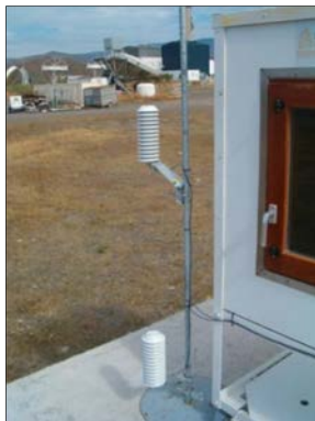
Figure 42: Meteorological sensors near the test box: Outdoors air temperature, global vertical solar radiation, wind speed and direction.
