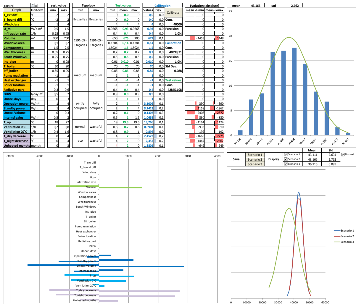
Figure 6.4 General view of the simulation-based evaluation tool developed to analyze residential building design: Upper left: input of parameters bounds and values Upper right: performance of one design as a statistical distribution curve Lower left: sensitivity of the performance to each input parameter Lower right: comparison of three scenarios
