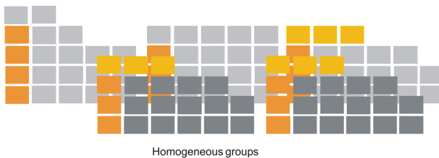
Figure 5-12: The orange marked apartments have one dominating homogeneous specification: the orientation (dark orange on the left side) and structure type (light orange on top floor as lightweight construction).
