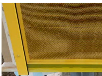
Figure 9: Solar comb protected by a toughened glass panel
