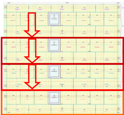
Figure 17: Sequence of assembly of the façade modules (Source view: Kulmer Bau)
