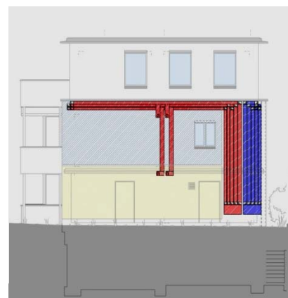
Figure 16: Ventilation distribution on north-east façade
