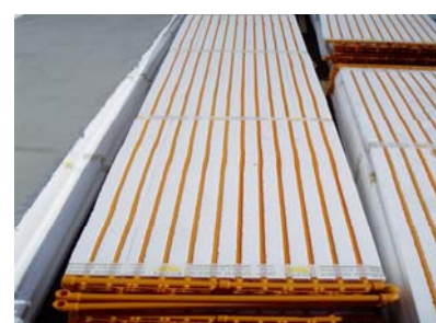
Figure 17: Heating pipes are inserted in XPS insulation boards.
