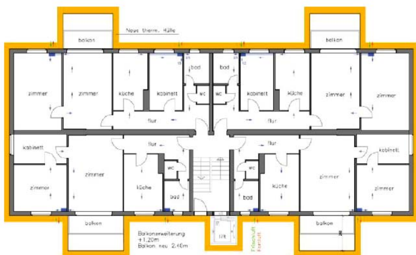
Figure 5: Exemplary floor plan of renovated building – showing new thermal envelope, integrated balconies and new lift (Source: Hohensinn ZT GmbH).
