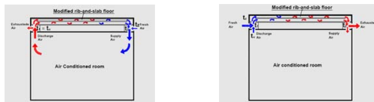
fig. 4: Air conditioning system based on thermal energy storage in building structure, night and day behaviour.
