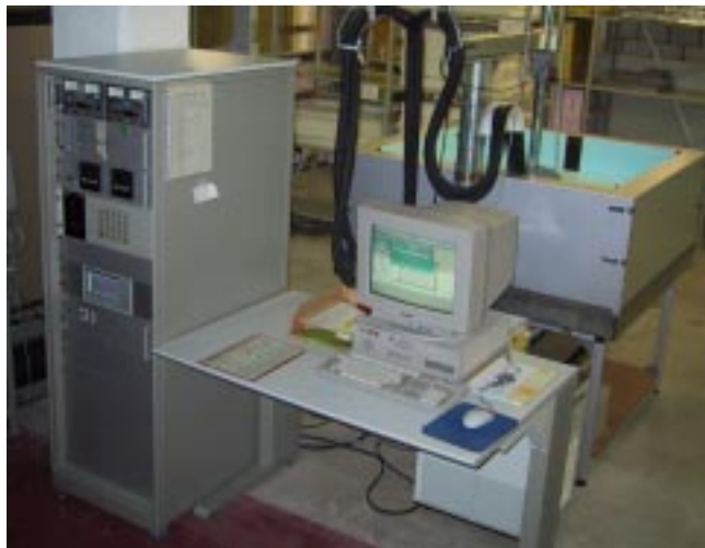
Fig. 2: One of EMPA's symmetric guarded hot plate facilities for low conductivity measurements on thermal insulation products (specimen size 750 x 750 \text{mm}^2 ).
