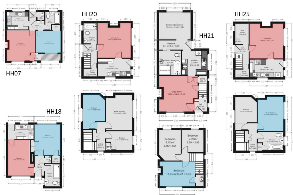
Figure 47. Layouts of the SMETER test cases. For each dwelling, the living room is shown in red and the main bedroom in blue.
