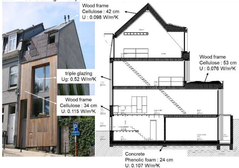
Figure 17. Uccle Test House: East façade and cross-section (source: Atelier d'architecture Gérard Bedoret).
