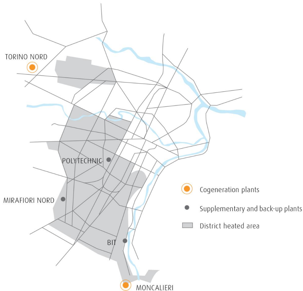
Figure 1. Schema of Turin District Heating Network, showing the two main stations and the supplementary substations for the heated area
