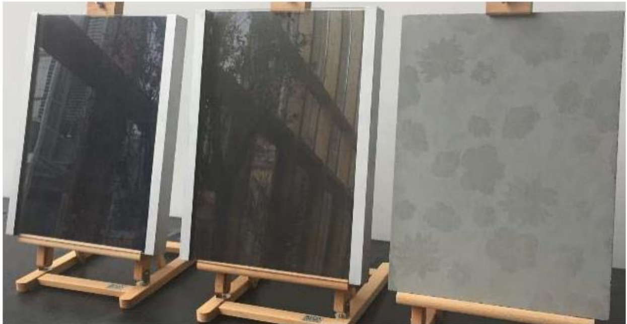
Figure 64. TABsolar panels (Source: [5]).
