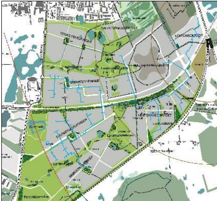
Figure 81. District cooling network from hydraulic analysis to all buildings that have a cooling demand (Source: Ramboll and Hillerød Municipality).
