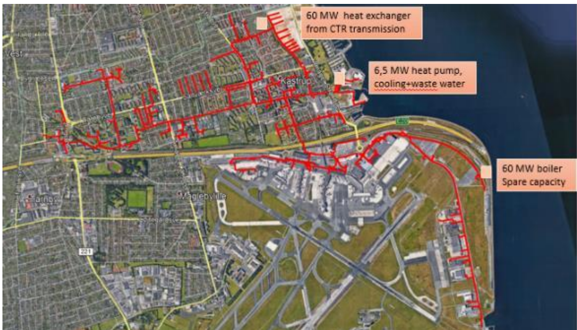
Figure 35. Trench of the network from the hydraulic model. Source: Taarnby Forsyning and Ramboll.
