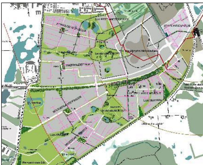
Figure 80. District heating network from hydraulic analysis in all districts (Source: Ramboll and Hillerød Municipality).
