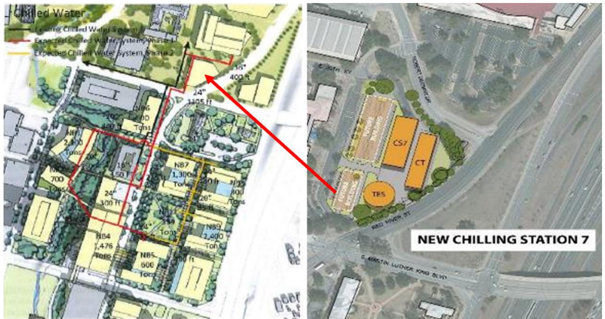
Figure 140. Chilled-water and heating water connections for the Medical District (Phase 1) at the University of Texas Austin and close up of new chilling station and thermal energy storage (TES) tank (Source: University of Texas Austin 2015).
