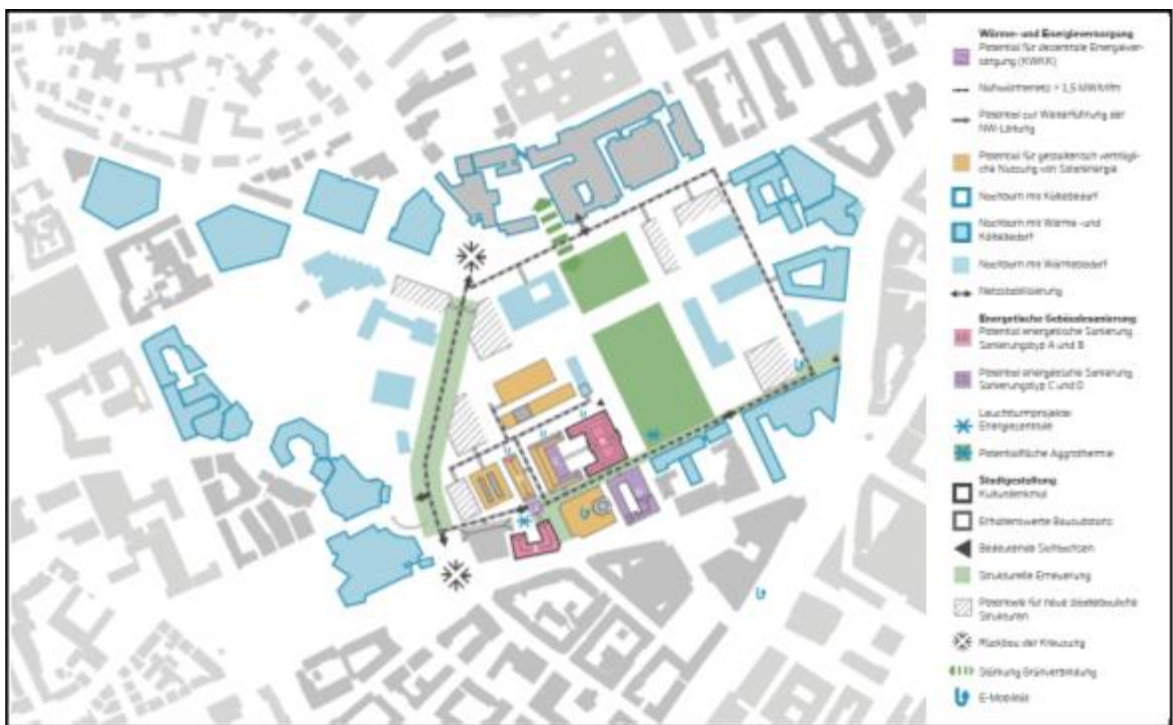
Figure 113. Concept of energy demand and distribution and refurbishment potentials in the Campus neighborhood (Source: Handlungsleitfaden – Energieleitplan | ZNS HFT Stuttgart).
